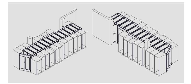
Using this modular system significantly increases the efficiency of the under floor cooling provided within the Data Centre. The cool air can now flow into the Containment area where it is drawn through the equipment and expelled out the rear, now the air is more effectively utilised. In some cases a reduction in the cooling energy within the data centre can be achieved.
